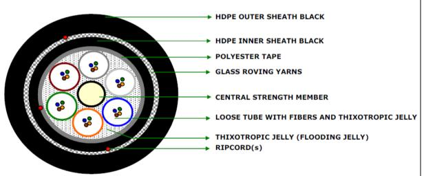
**3.8.1 Secondary Protection:** The primary coated fibres may be protected by loose packaging within tube, which shall be filled with thixotropic jelly. The dimensions of tube shall be as per Annexure – I.
